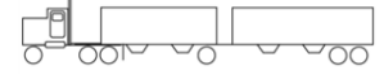
Truck Tractor / Semi Trailer / Semi Trailer (other combination) overall length limited to 65 ft. 8-1904(c)
